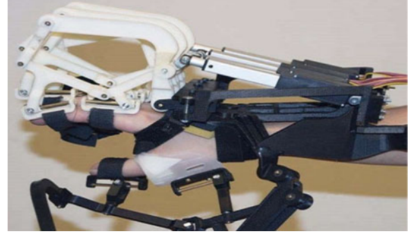
Fig. 3. Multi-fingered underactuated hand exoskeleton.
